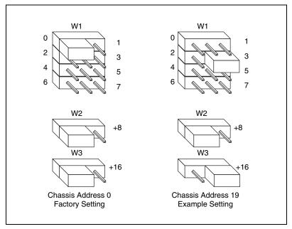
Figure 2-8. SCXI-1000DC Chassis Address Jumper Settings
